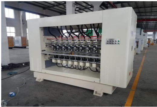
Electric adjusting knife, pneumatic lifting knife
