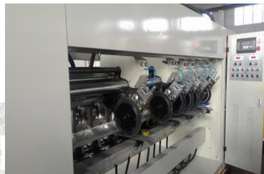
Up and down pressure line synchronous adjustment down pressure line can be fine-tuned
